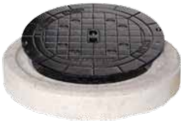
NEW! Combination cover round DN/OD 400 concrete and cast iron B125 (12,5 t), without ventilation
